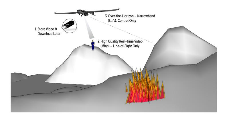
An advantage confined to large drones with large payload capacities has been the use of fast, secure satellite links to provide enough bandwidth (Megabits per second, or Mb/s) for high quality video to be delivered securely, and in real time. However, **the big problem is** that the equipment required to deliver high quality video over satellite is too large and too heavy to be flown on smaller drones.
