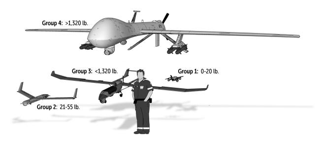
Even for the largest drones, size, weight, and power (SWaP) are critical, but for smaller Group 2 & 3 platforms, the pressure is magnified. Beyond the smaller available space and smaller payload capacity, smaller batteries mean less range unless the internal systems can be engineered to draw less power. It can also mean less ability to communicate.
